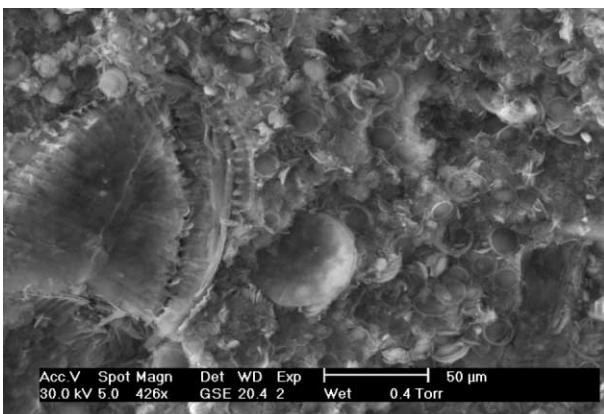
Plate 3. Progressive opal-A dissolution of large diatom frustules, Erdobenyne pure diatomite sample, Erdobenyne, Hungary.
