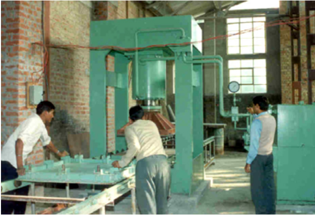
Fig. 2. 400 ton capacity hydraulic moulding press.
