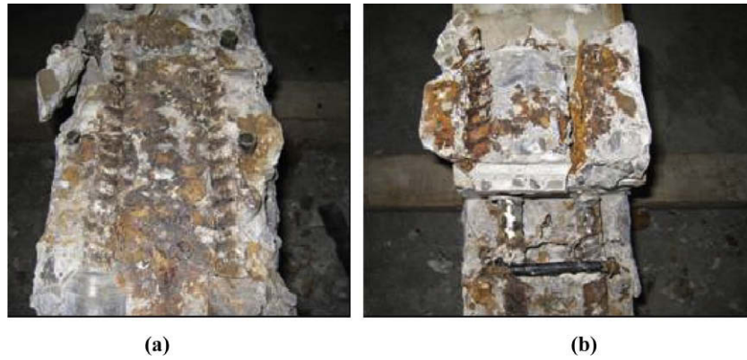
Fig. 11. Fatigue failure in beam F-U-43-I: (a) upper concrete above bar and (b) lower concrete below the bar.
