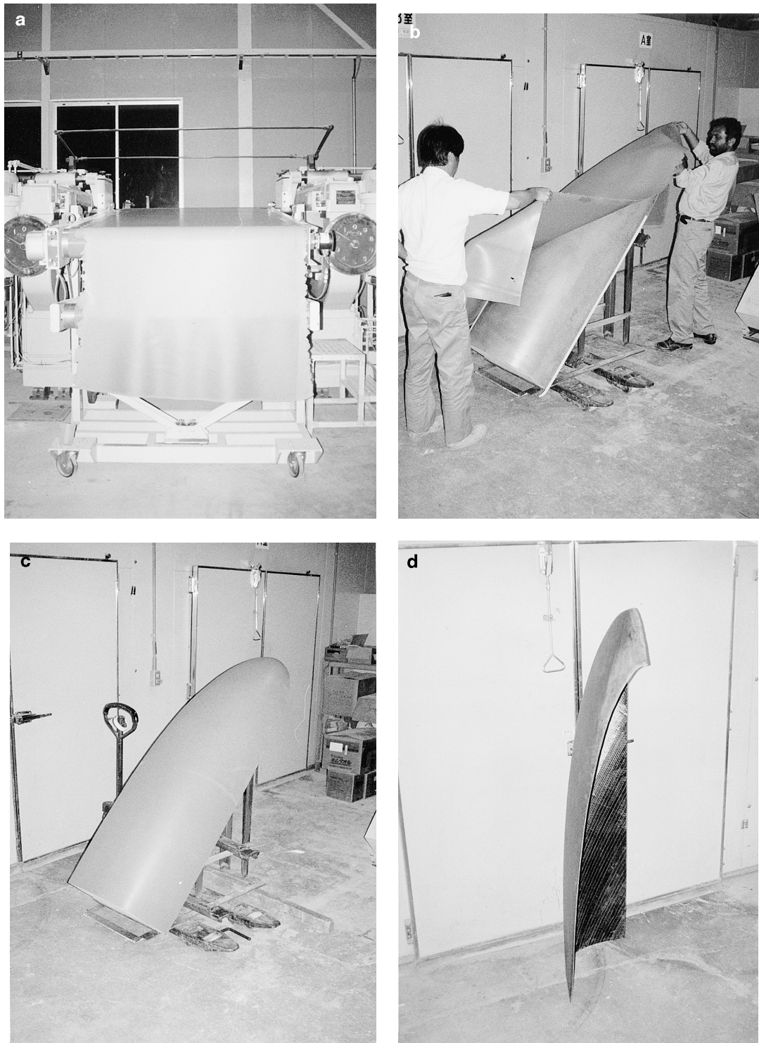
Fig. 11. Various steps in making a cement shell. (a) A roller milled sheet positioned on a conveyor belt. (b) Shaping using a previously made concrete mold. (c) The sheet adhered to the concrete mold. (d) The final product.
