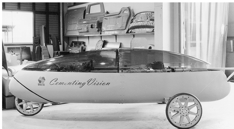
Fig. 10. View of the solar-powered car in which the body is made by the CAPR composite.
