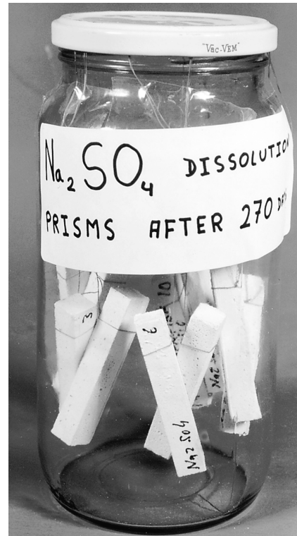
Fig. 1. Photograph of prisms after 270 days in Na 2 SO 4 solution.
