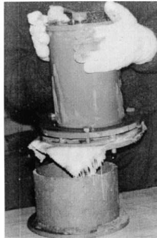
1 – manometer 2 – orifice for compressed air 3 – orifice for concrete filling 4 – concrete or cement paste 5 – fabric 6 – tank for collecting the drained liquid
