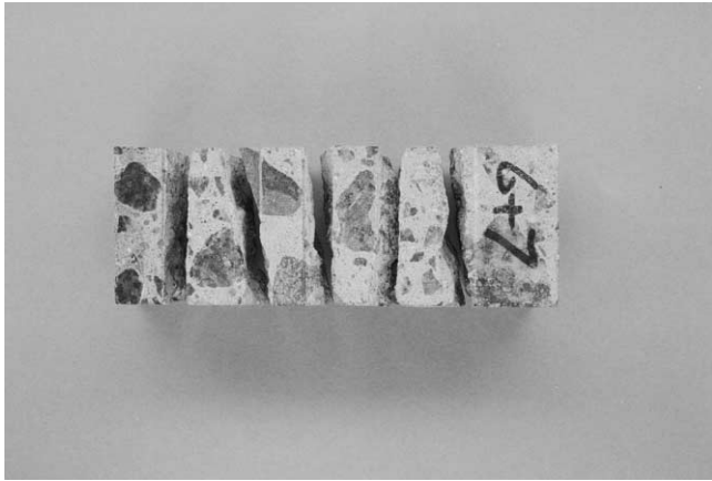
Fig. 1. Subdivision of prisms for determination of moisture content.
