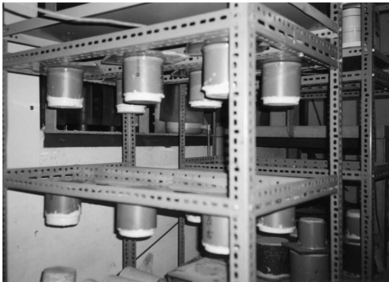
Fig. 3. Salt ponding test setup showing concrete specimens encased in PVC pipes.
