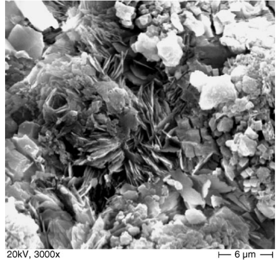
Fig. 8. Micrograph showing plate-like gypsum crystals. Aerial lime based mortar.
