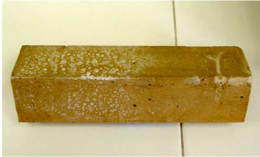
Fig. 7. SO 2 alteration in a hydraulic specimen.
