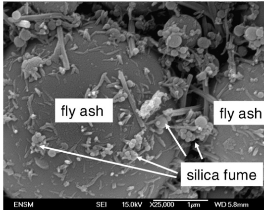
Fig. 8. SEM-micrograph of a silica fume containing fly ash based mortar taken after 24 h of curing.
