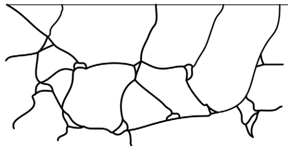
Fig. 8. When there is no crack, the slip planes are constrained by the intergranular phase.
