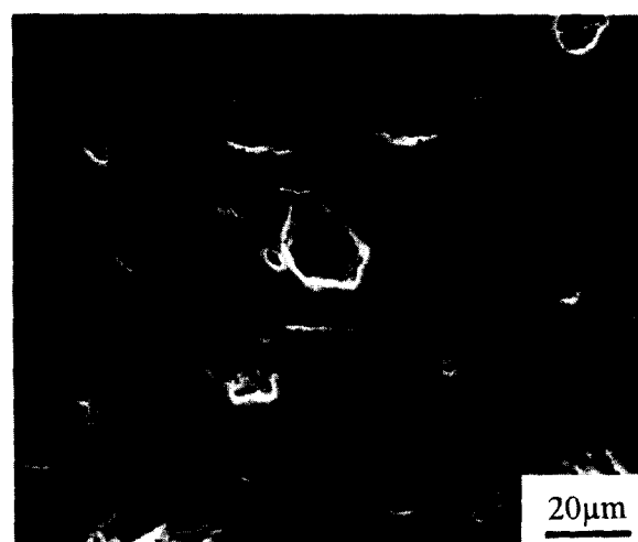
Fig. 5. An SEM micrograph from the cross-section of a 20 vol.% SiC platelet reinforced 3Y-TZP composite, revealing crack-like voids and porosity associated with platelets as shown by arrows.
